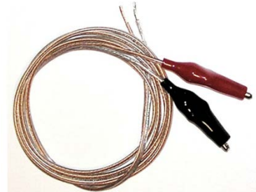
Figure 3.2-3: Completed Power Cord
