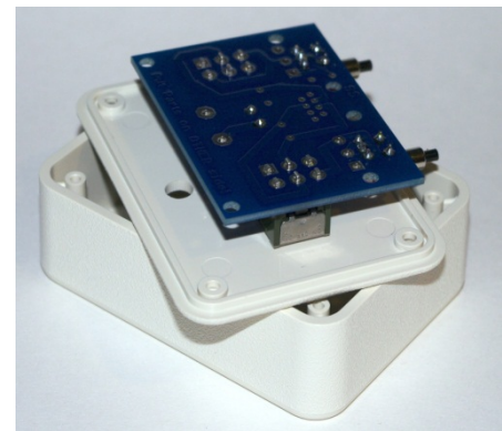
Figure 3.3-4: Toggle Switches Held Straight by the Control Box Lid During the Soldering Process
